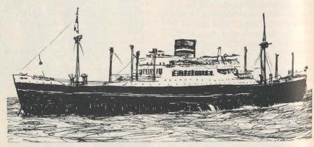
Cargo-Passenger: this ship is equipped with cargo handling facilities as well as passenger accommodations.
